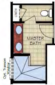
OPT. L-SHAPED SHOWER LAYOUT WITH ZERO THRESHOLD
