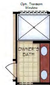
OPTIONAL UNIVERSAL SHOWER LAYOUT WITH ZERO THRESHOLD
