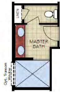
OPT. UNIVERSAL SHOWER LAYOUT WITH ZERO THRESHOLD
