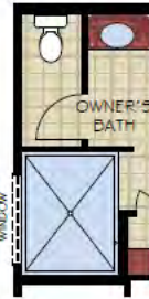
OPTIONAL UNIVERSAL SHOWER LAYOUT WITH ZERO THRESHOLD
