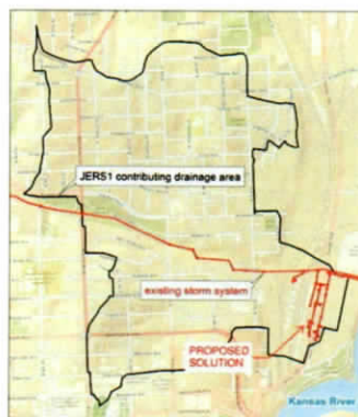
Figure 1-6 JERS-1 Existing Stormwater Network
