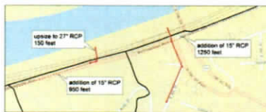
Figure 1-5 ARGE-1 Proposed Stormwater Network (East Section)
