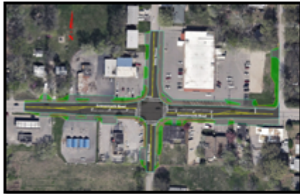
Above: showing the addition and redesign of green space, sidewalks, and new signals at the intersection of 55 th St and Leavenworth Rd.
