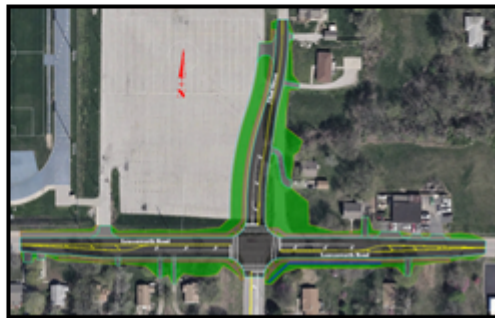
Right: Design rendering showing the realignment of the intersection at 72 nd St and Leavenworth Rd. Realignment will allow for proper turn lanes, new signals, and pedestrian walk ways.
