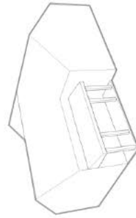
Shed Roof Front Porch
