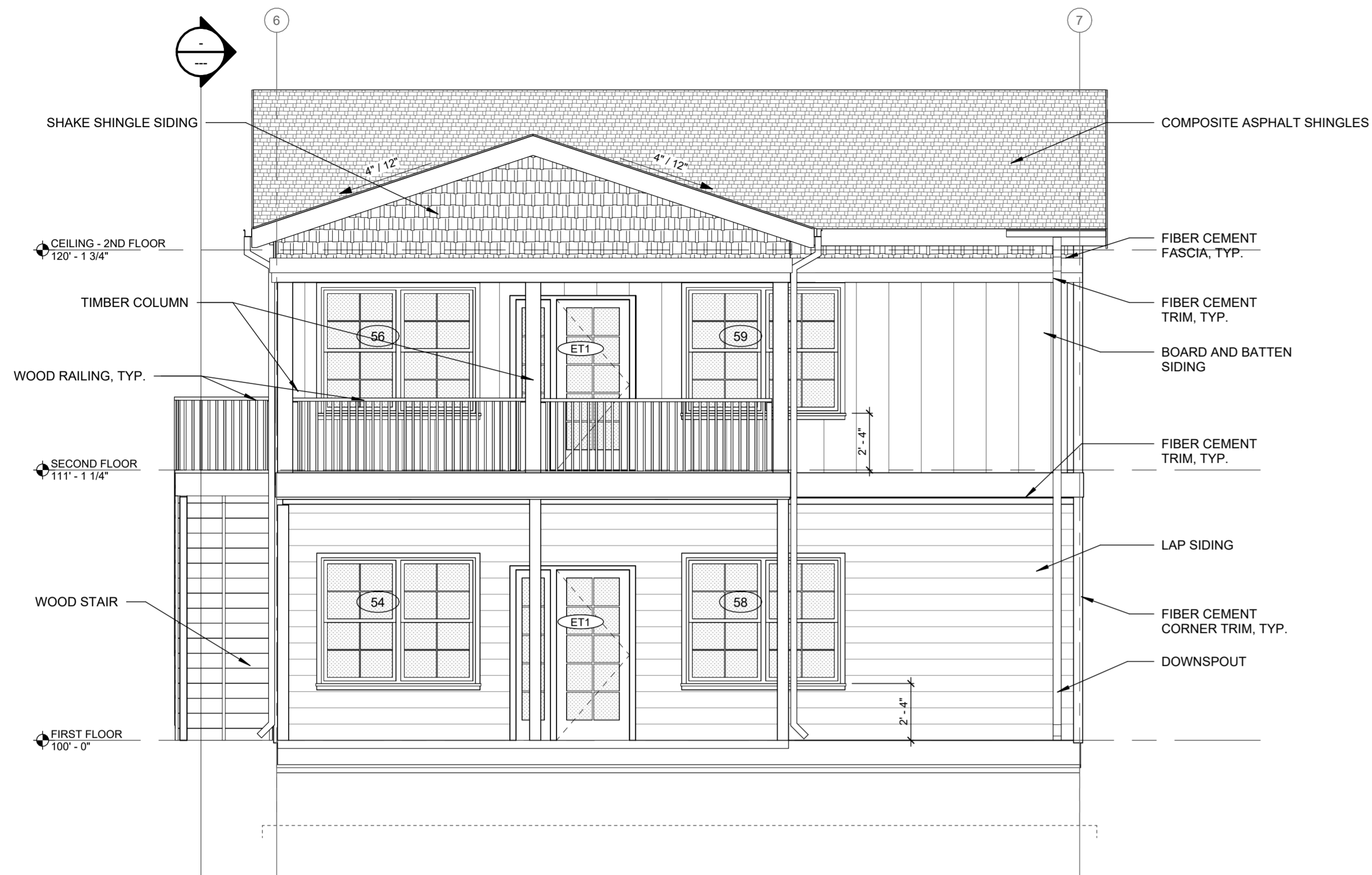
1 DUPLEX SINGLE - FRONT ELEVATION 1/4" = 1'-0"
