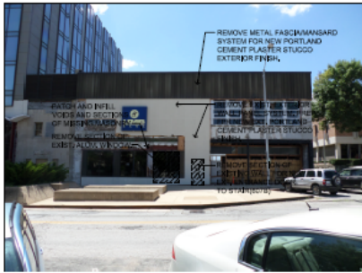
1 EXTERIOR WALL DEMOLITION NO SCALE
